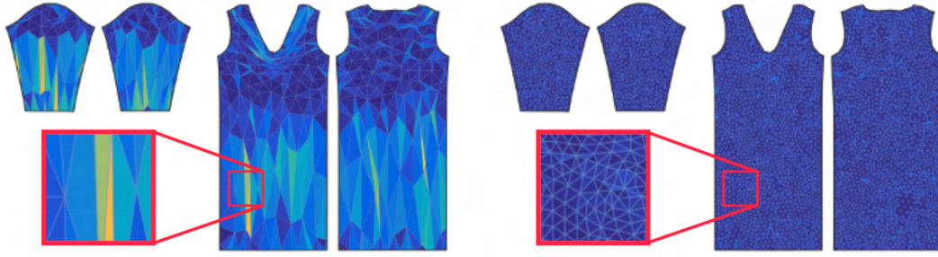
Figure 4.6: Garment type-dependent topology optimization, here shown in 2D panel space. Left: the 2D layout of a long dress design, with the template topology \bar{\mathcal{T}} . Right: the same design after the topology optimization step, resulting in the mesh \bar{\mathcal{M}} with homogeneous triangle size and without degenerated geometry.
