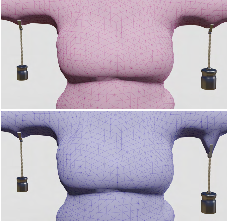
Figure 3.5: This picture shows the deformation of our material (top) in comparison with the nonlinear flesh material defined in [SGK18] (bottom), for two different weights under gravity: 0.5Kg (left) and 2.0Kg (right). It can be clearly seen that our material provides a higher nonlinear response.
