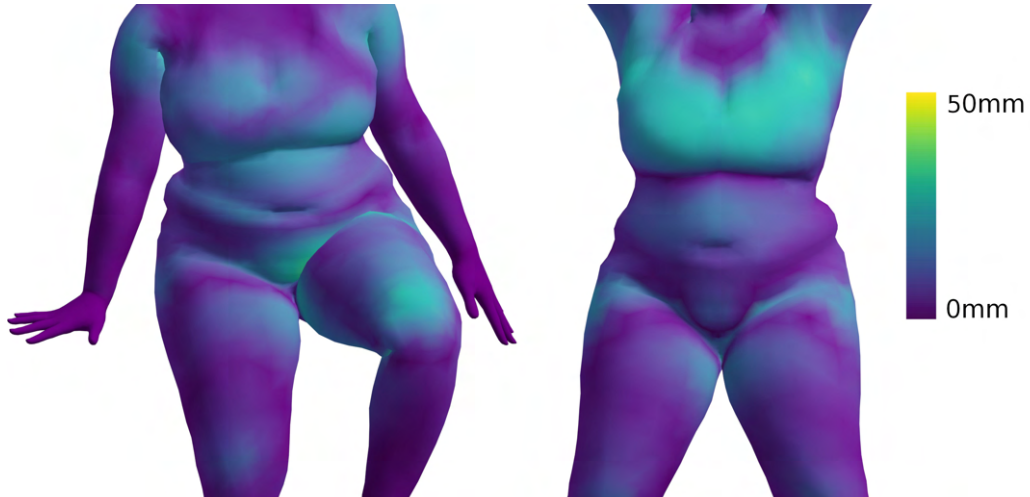
Figure 3.4: This picture shows the resulting deformation for two static poses when defining the deformation gradient in world space as in [Kim*17]. The color map highlights where the result differs from the data-driven static deformation of SMPL.
