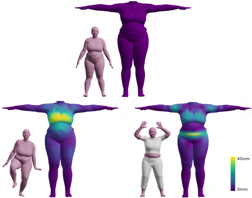
Figure 3.2: These are three examples of posed avatars (inset) subject to various soft-tissue deformations expressed in unposed space through a color map. For a static pose (top), the unposed shape is undeformed and identical to the reference shape. For highly dynamic (left) or external interaction (right) scenarios, the unposed shape shows high-frequency local deformations.
