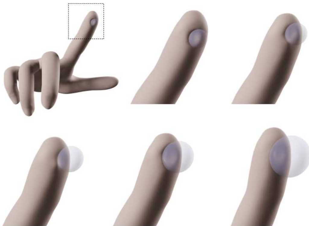
Figure 4.12: We model a finger with just 3 frame handles located at the phalanges. The full nonlinear deformation of the surrounding tissue is captured by our learning-based corrections. Moreover, in this example we learn external corrections as a function of the size of the spherical collider, opening the possibility of using parametric shape models.
