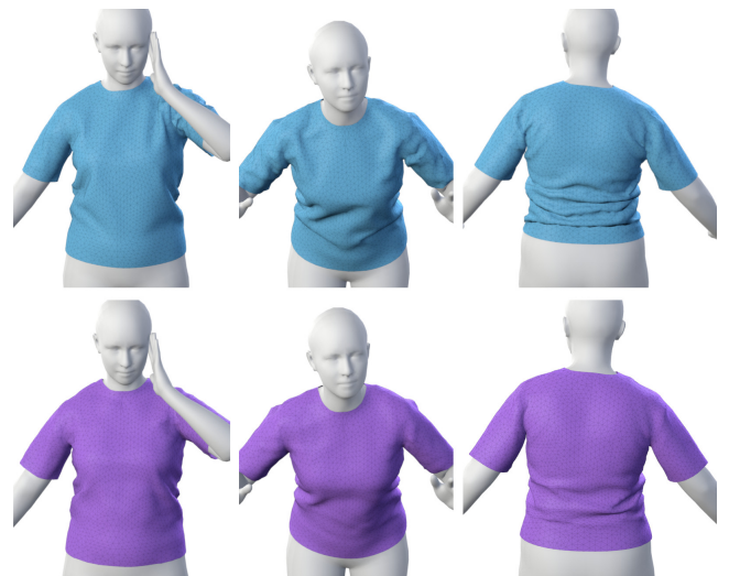
Figure 11: Comparison between a ground-truth physics-based simulation (top) and our data-driven method (bottom), on a test sequence not used for training (01_01 from [CMU]). Even though our method runs three orders of magnitude faster, it succeeds to predict the overall fit and mid-scale wrinkles of the garment.
