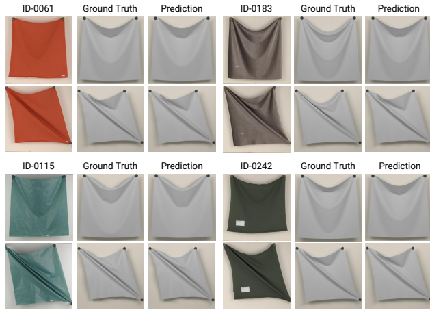
Figure 10: A comparison between the simulations obtained through the ground truth parameters, and those obtained using the predictions of our model, from a representative set of fabrics of our test set. As shown, the estimations of the model yield similar drapes to those of their ground truth counterparts, which we also evaluate quantitatively.
