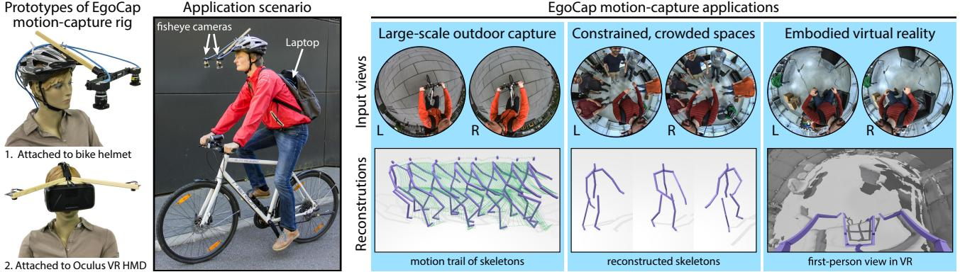
**Figure 1:** We propose a marker-less optical motion-capture approach that only uses two head-mounted fisheye cameras (see rigs on the left). Our approach enables three new application scenarios: (1) capturing human motions in outdoor environments of virtually unlimited size, (2) capturing motions in space-constrained environments, e.g. during social interactions, and (3) rendering the reconstruction of one’s real body in virtual reality for embodied immersion.
