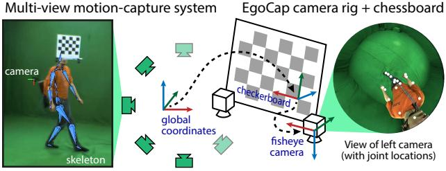
**Figure 3:** For database annotation, the skeleton estimated from the multi-view motion capture system (left), is converted from global coordinates (center) into each fisheye camera’s coordinate system (right) via the checkerboard.
