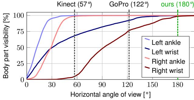
**Figure 6:** Visibility of selected body parts for different camera angles of view, for the left-hand camera in our rig over a 5-minute recording. Seeing the right wrist 95 percent of the time requires an angle of view in excess of 160°, which is only practical with fisheye lenses.
