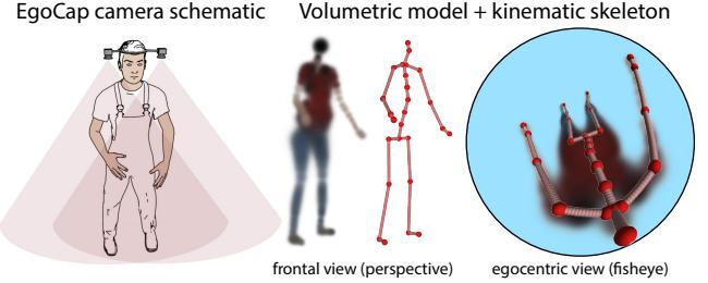
**Figure 2:** Schematic of EgoCap, our egocentric motion-capture rig (left), visualization of the corresponding volumetric body model and kinematic skeleton (center), and the egocentric view of both in our head-mounted fisheye cameras (right).
