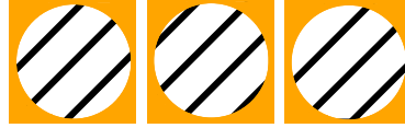
Figure 3.14: Aperture problem: it is not possible to know how the lines are moving just looking through the hole. To know the correct answer it is necessary to see the end of the lines.
