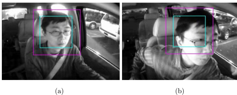
Figure 6.1: Example showing the importance of the scale factor. In this sequence the tracked face comes closer to the camera, but the square that shows where the face is keeps the same size. A tracker method that contemplates the scale factor, would increase the size of the square.
