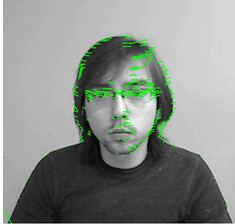
Figure 5.9: Optical flow of the good features to track between the first and the tenth frame of the sequence shown in Figure 5.8. In this sequence the subject is moving his face to the left, as the optical flow vectors shows.
