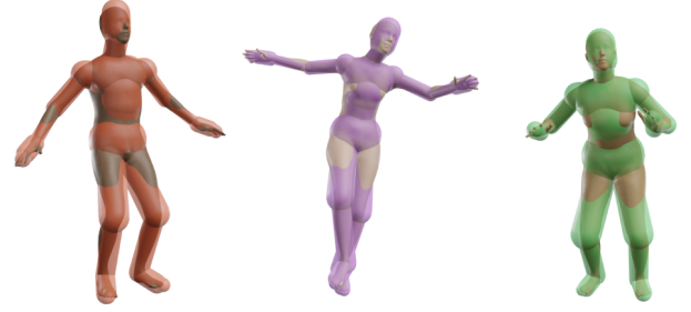
Fig. 2. Three example poses of our underlying 3D body representation. We enrich the SMPL [Loper et al. 2015] parametric human model (in solid brown) with a set of parametric volumetric 3D primitives (in semitransparent colors), which enables fast and highly efficient evaluation of collisions.
