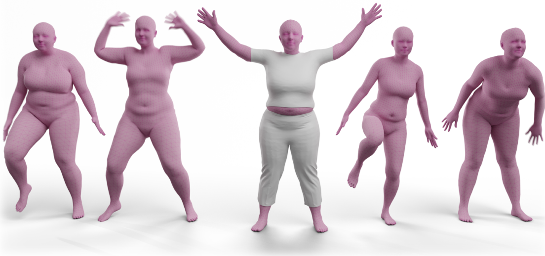
Figure 1: Our soft-tissue avatar combines a statistical model and an FEM simulation. Our custom constitutive material produces highly dynamic effects and realistic external interactions. We characterize material parameters to match 4D captures using numerical optimization.
